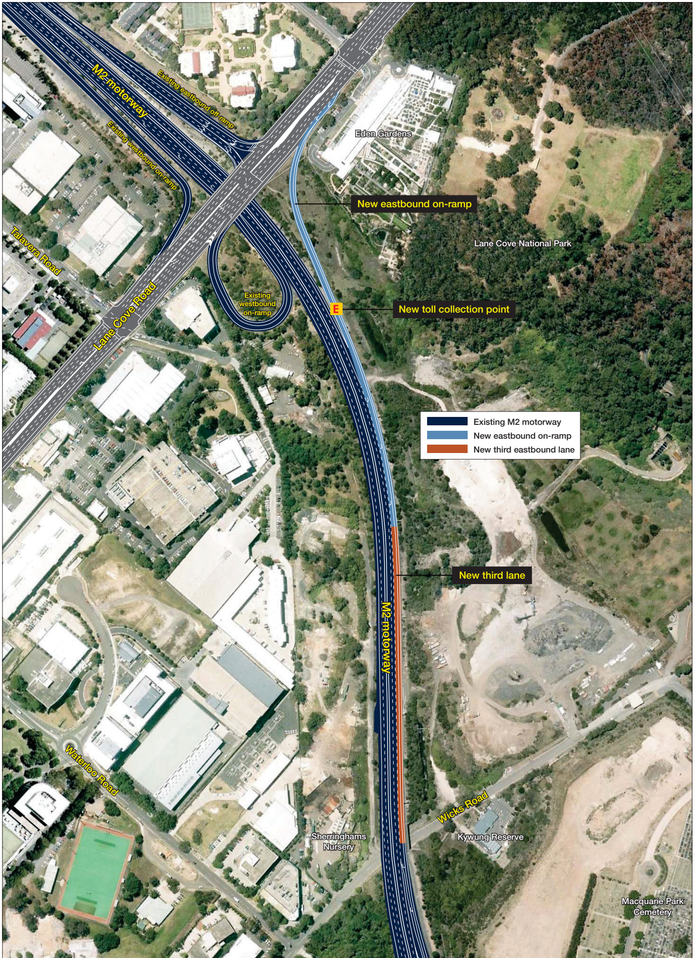
Figure 1.5. The new eastbound on-ramp from Lane Cove Road to the M2 motorway in Macquarie Park.
