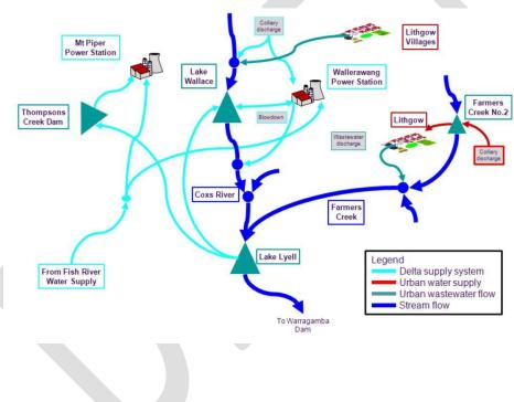
Figure 6.1 Schematic of Coxs River Water Supply (SKM, 2011)
